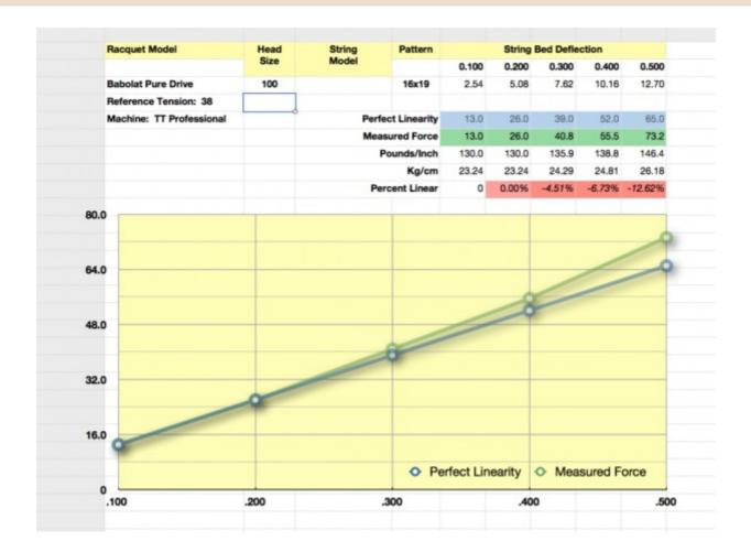
But for a string bed with low elongation strings (less than 5%) under low pulled tensions (less than 20 lbs., or tensions that have been reduced due to racquet deformation and/or string tension relaxing with time), the SBS additionally depends on the string elongation and will significantly increase, in a nonlinear ever-increasing way, for harder ball impacts.
