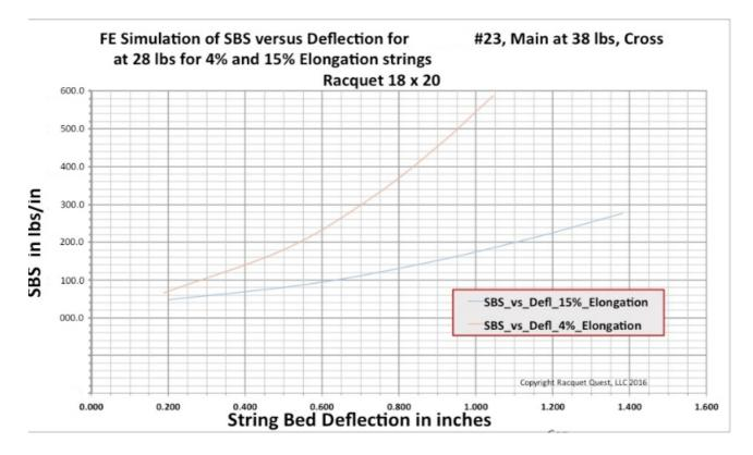
As you can see by the graph, elongation contributes to SBS in a big way. The red line indicates a stiff string, about 4%, and the blue line indicates a "soft" string, about 15% elongation. You can see the loads increase dramatically as the impact increases. So the harder the hit the higher the loads on the body.
